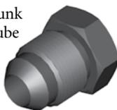
No. 6 JIC (9/16" x 18NF) male braze-on fitting for power steering tubes.
