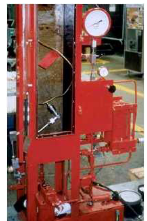
Figure 4. Equipment used to test hydrostatic pressure in brake tube.
