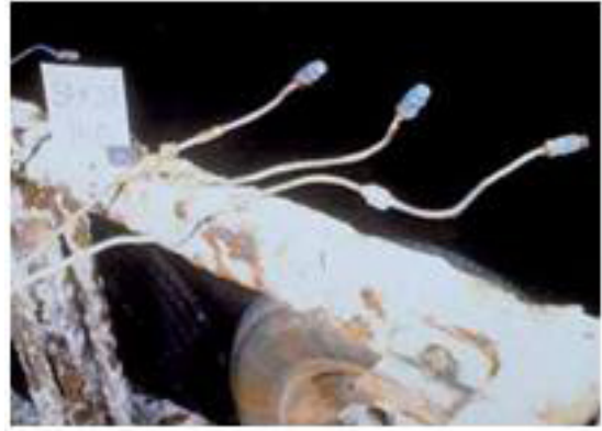
Figure 3. Brake line samples attached to test trailer.
